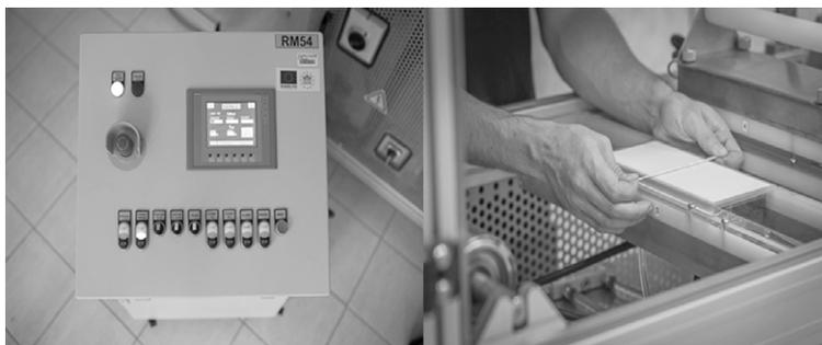
Fig. 2. Panel with control unit (left) and flat electrode (right)
