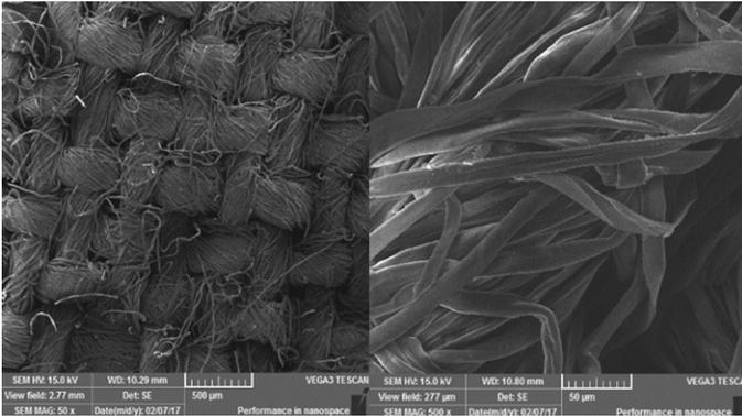
Fig. 4. SEM images of untreated cotton fabric 50x (left) and 500x (right)
