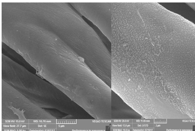
Fig. 7 SEM images of untreated cotton fabric (5kx, left) and plasma-treated cotton fabric at 375 W, 35 s (10kx, right).
