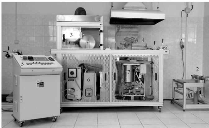
Fig. 1. Description of plasma laboratory equipment KPR 20 – 1 Reel-off unit; 2 Take-up unit; 3 Concave curved electrodes; 4 Flat electrodes; 5 Control unit; 6 H-V power supplies; 7 Oil based cooling system.
