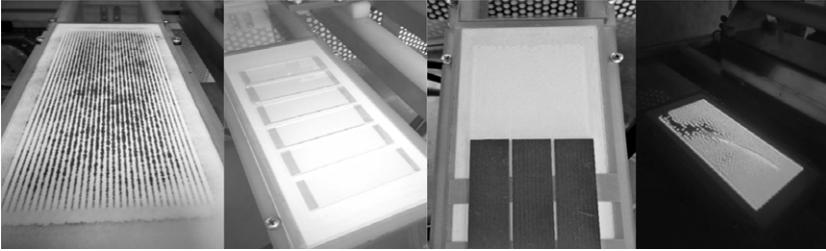
Fig. 3. Materials which can be used for DCSBD plasma treatment (powder, glass, textile)
